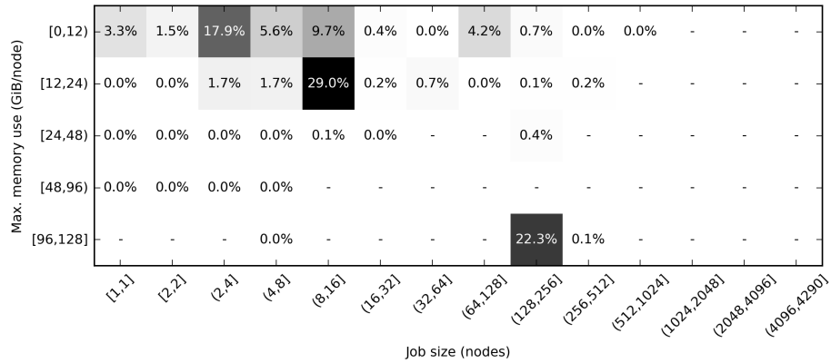
Fig. 4. Usage heatmap of maximum memory versus job size for Met Office UM jobs in the period.
