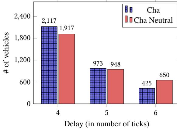
Fig. 7. Benefit from prosociality. Delays ( $\geq 4$ ) with Cha Neutral and Cha. 35% of vehicles that experience the highest delay (6 ticks) with Cha Neutral experience an improvement of  $\geq 16.67\%$  with Cha.
