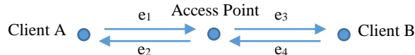
Figure 1. Simple network setup. Each client A and B is connected to the access point by two directional edges e_1, e_2, \dots, e_4 .
