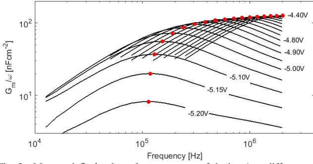
Fig. 2. Measured  $G_m/\omega$  through gate contact of device A at different gate voltages, peak positions are marked with circles.  $f_{gc}$  falls and then becomes constant at -4V, following the behavior of mobility.
