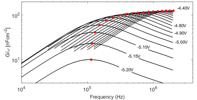
Fig. 3. Modelled  $G_m/\omega$  through gate contact of device A at different gate voltages, peak positions are marked with circles.  $f_{gc}$  has been fitted to measurements in Fig. 2 using mobility as the only free parameter, thus extracting the mobility.
