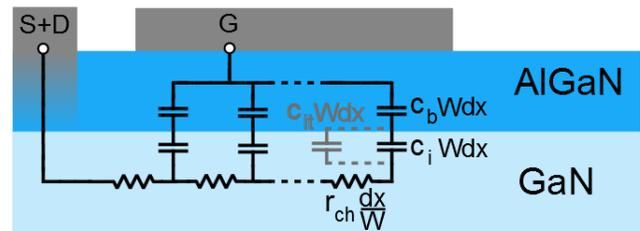
Fig. 1. Equivalent circuit model of fatFET capacitor structure. The device is of length  $L = \sum dx$  and width  $W$ .  $r_{ch}$  is the sheet resistance,  $c_i$  is the capacitance per unit area of the 2DEG,  $c_b$  is the barrier capacitance per unit area. The capacitance per unit area of interface traps,  $c_{it}$  is depicted greyed on the figure, but is not included on the model as it is not the dominant loss mechanism for large gate length devices such as the one considered here.
