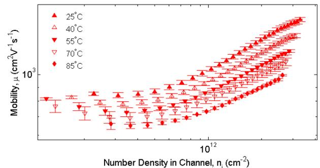
Fig. 6. Extracted mobility for device C at different temperatures. The mobility decreases at all electron concentrations as temperatures rises. At high electron concentrations  $> 10^{12} \text{ cm}^{-2}$  the power law dependence ( $\mu \propto n_i^\gamma$ ) changes such that  $\gamma$  decreases by 17% at 85°C. This indicates an increased contribution of phonon scattering to the mobility.
