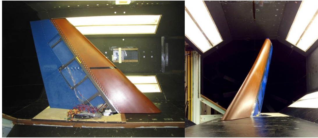
Figure 3. Assembly process of the wingtip in the wind tunnel (left) and assembled model at -10^\circ angle of attack (right).
