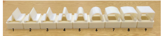
Fig. 6. The 9 stimuli used in this experiment, ranging in spatial scale from an edge (1) to flat surface (9) with intermediate curvatures ranging from 0.8 (2) to 0.0125 (8). The sensor travels ( y ) from right to left on each stimulus, covering 30 mm symmetrically about the apex of the stimulus.
