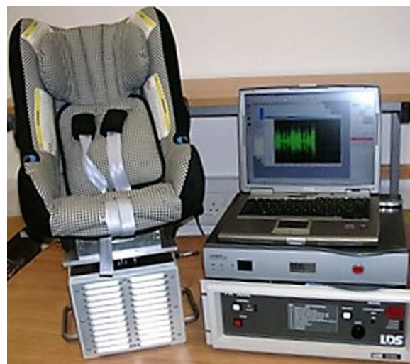
Figure 1 Car seat motion simulator with controls.
