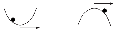
FIG. 7. The two different states that drive the orientation of the dipole. The left figure displays the stable state where the system is pulled by the minimum of the potential. The right figure displays the unstable state where the system is pushed by the maximum of the potential.
