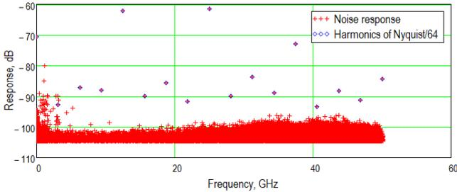
Fig. 3. Noise response of 50 GHz, 200 GSa/s DRTO showing the sub-Nyquist noise spurs corresponding to 64 ADCs
