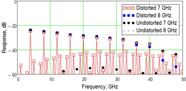
Fig. 2 IQ reference distortion creates IM products on the measured comb waveform. Choice of IQ frequency is important to avoid systematic errors.
