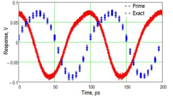
Fig. 4. Distorted waveform from an amplifier measured using the exact target frequency the prime-number sampling strategy.
