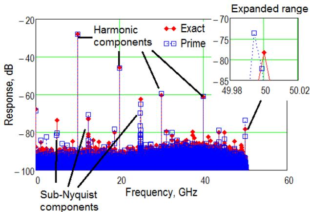
Fig. 5 Frequency components of the distorted signal show good agreement for the two sampling strategies except at 50 GHz.
