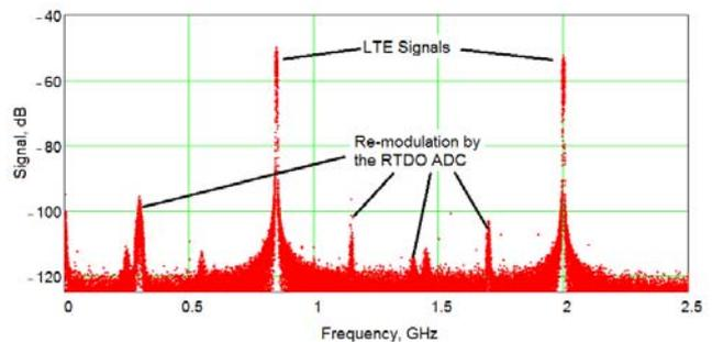
Fig. 6. Frequency components of the LTE waveform showing signal components and DRTO artifacts.
