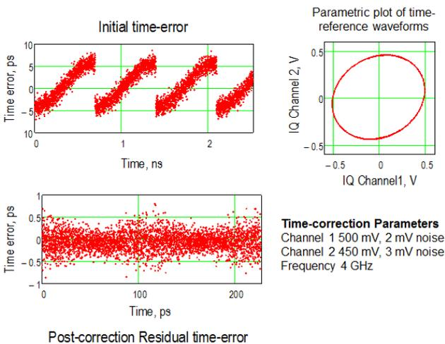
Fig 1. In-phase and quadrature (IQ) timebase correction using simulated data with unequal channel noise. The timing errors are reduced to the sub-picosecond level but the residual timing errors show periodic modulation at the IQ frequency.
