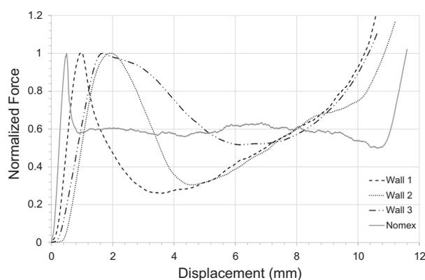
**Figure 5** Normalized force–displacement curves for ABS printed cores (dashed lines) and the Nomex honeycomb core (solid line). The force is normalized to the ultimate load to show the varying failure behaviors between core types
