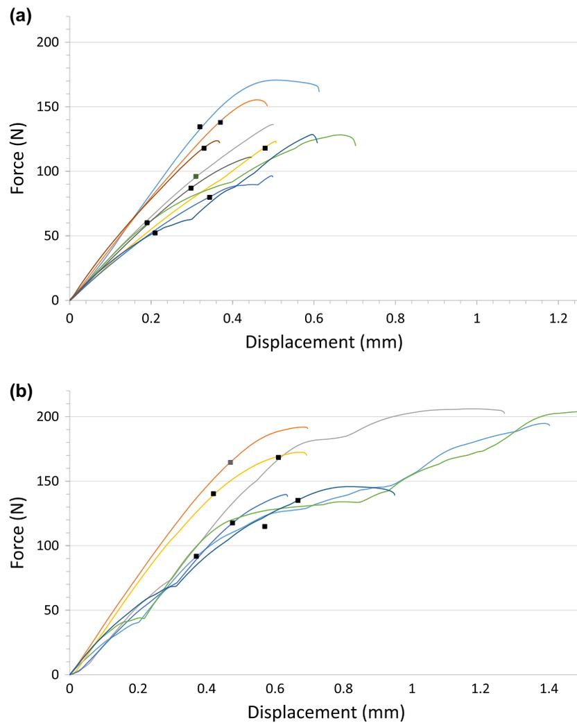
**Figure 8** Force–displacement curves for PLA tensile specimens printed with differing layer times. The black squares represent the yield points of the specimens, found through observation of the end of the elastic region of the force{displacement curve. (a) was printed with the same parameters as Figure 7a, while (b) had a 13 s pause applied
