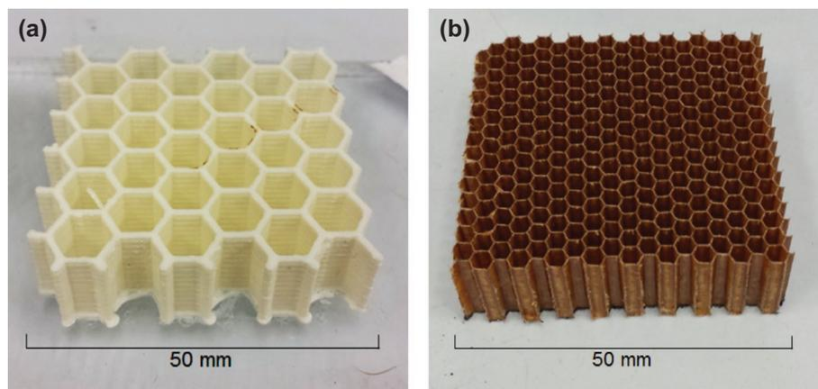
**Figure 4** Cores used during testing. (a) An example core of ABS manufactured through FDM, as used within this paper. (b) A Nomex honeycomb core of the same size; the difference in cell size due to the manufacturing limitations of the FDM process is clear
