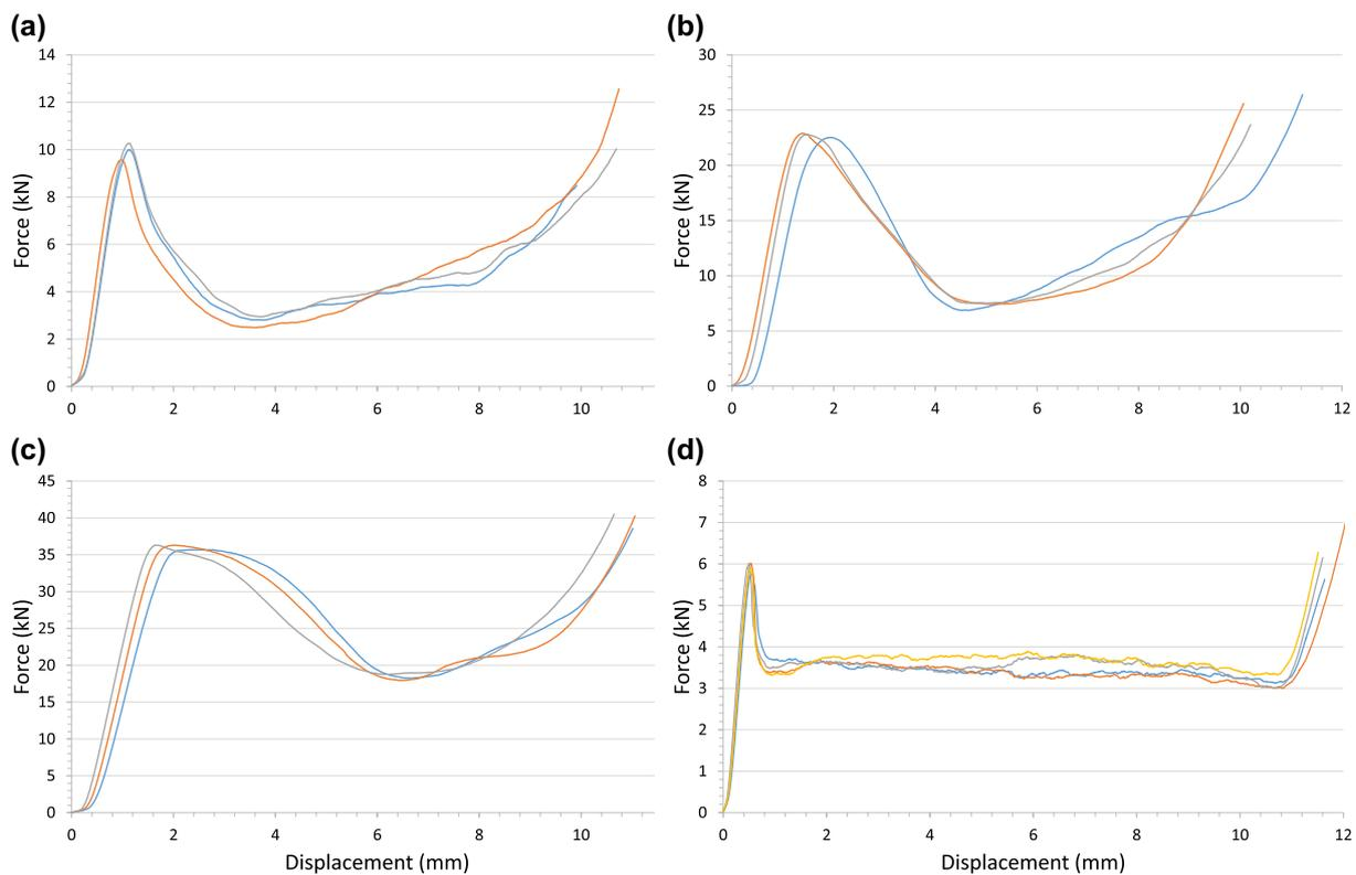
**Figure 9** Force–displacement curves for compressive testing of ABS cores produced through Fused Deposition Modeling (FDM). (a) was manufactured using toolpath 1, as described in Figure 3. (b) and (c) were manufacturing using toolpaths 2 and 3 respectively. (d) is a Nomex honeycomb core, with a cell size 3.2 mm and density  $48 \text{ kg m}^{-3}$ , commonly used within the aerospace industry
