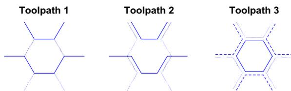
**Figure 3** The pictorial representation of the three toolpaths investigated, depicted for the construction of a single hexagon cell. The lines are offset to show each pass on for the edges of the honeycomb cell. Each line of continuous extrusion is represented by a different dash type.
