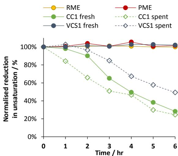
Figure 7. Normalised reduction in unsaturation calculated from the <sup>1</sup>H NMR of the biodiesel samples held at 110 °C under a constant airflow
