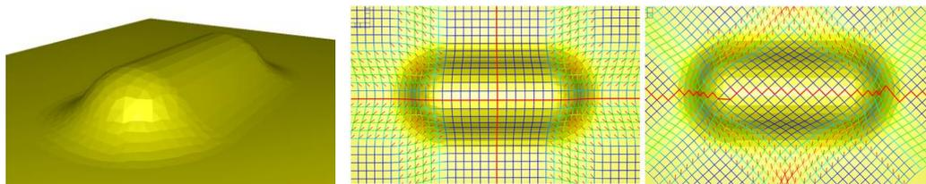
Figure 1: Schematic of how plies can shear over the mould shape generated using ‘Virtual Fabric Placement’ [ 8 ].(Left) Image of the formed shape (Middle)  $0^\circ/90^\circ$  orientation, (Right)  $\pm 45^\circ$  orientation.
