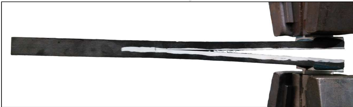
Figure 2. Carbon/epoxy laminate specimen undergoing static crack growth via DCB testing. The dimensions of the specimen are approximately 220 \times 25 \times 10 mm.
