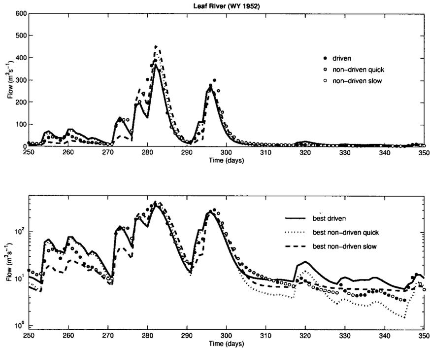
Fig. 11. Hydrograph range produced by the 500 Pareto solutions (grey region), and the output from the best parameter sets for the different measures on normal (1<sup>st</sup> row) and on logarithmic scale (2<sup>nd</sup> row). The observed time-series is shown as circles.
