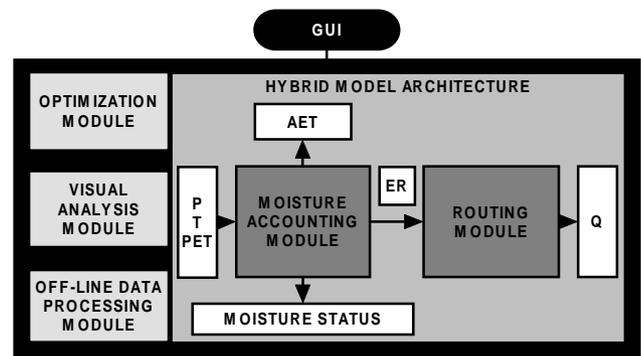
Fig. 3. The system architecture of the Rainfall-Runoff Modelling Toolbox (RRMT). The input and output variables shown in the figure are: the precipitation  $P$ , the temperature  $T$ , the potential evapotranspiration  $PET$ , the actual evapotranspiration  $AET$ , the effective rainfall  $ER$ , and the simulated streamflow  $Q$ . The user can access the model via a Graphical User Interface (GUI).
