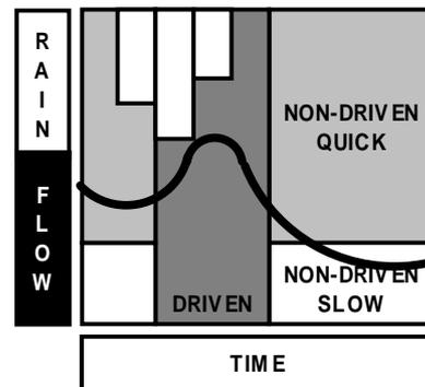
Fig. 5. Hydrograph segmentation into three components based on different response modes of the catchment system, i.e. “driven” ( $Q_D$  - dark grey), “non-driven quick” ( $Q_Q$  - light grey) and “non-driven slow” ( $Q_S$  - white) flow.
