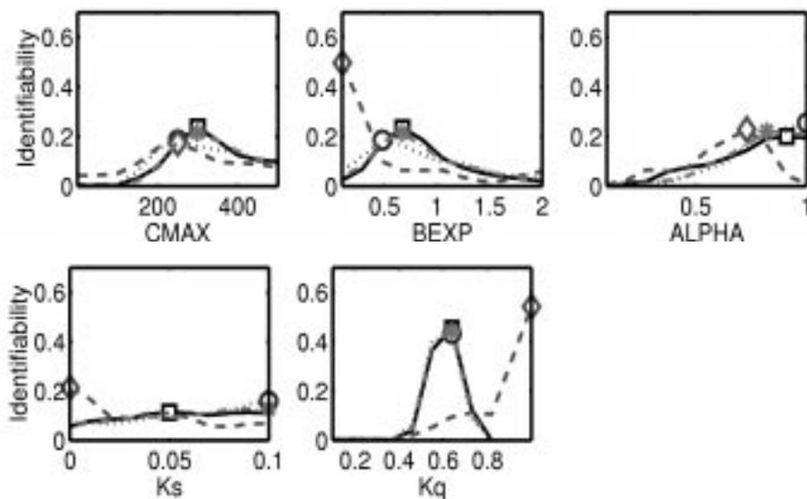
Fig. 9. The distribution of gradients for the different parameters and the different objective functions is shown. The markers indicate the highest gradient values for FD (rectangle), FQ (circle), FS (diamond) and RMSE (star), also ranging from dark (FD) to light (RMSE) grey shading.
