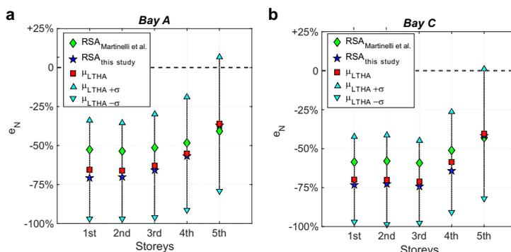
Fig. 4. Relative difference of design axial load ( $e_N$ ) for braces at each storey between RSAs and LTHA with respect to static analysis for (a) Bay A in x direction and (b) Bay C in y direction. For the case of LTHA the mean and the mean  $\pm$ one standard deviation is shown.
