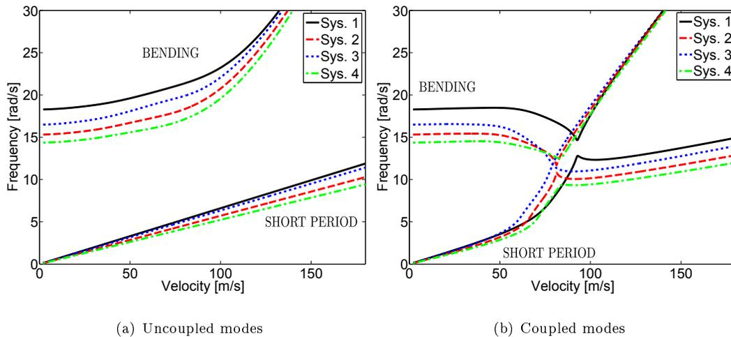
**Fig. 11 Physical BFF modes reconciliation: frequency vs velocity**
