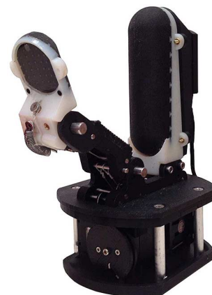
Fig. 1. TacThumb base mounted on the Open-Hand model M2 robotic gripper.
