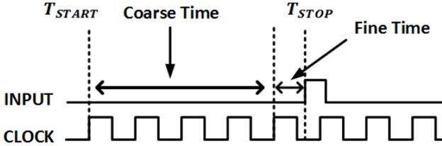
Fig. 3: Illustration of Nutt Interpolation
