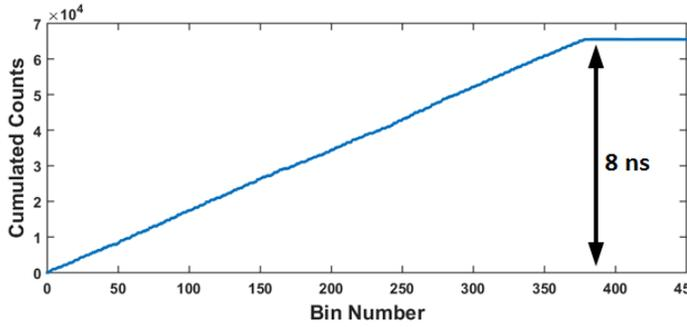
Fig. 8: Cumulative distribution of counts across delay-line structure
