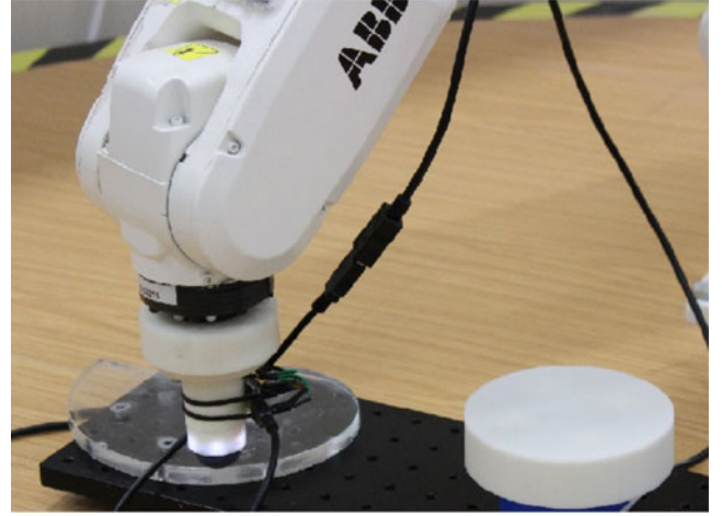
Fig. 3. Sensor mounted as an end-effector on the robot arm used for experiments. The two stimuli used are also shown: circle (right) and non-uniform volute (left).
