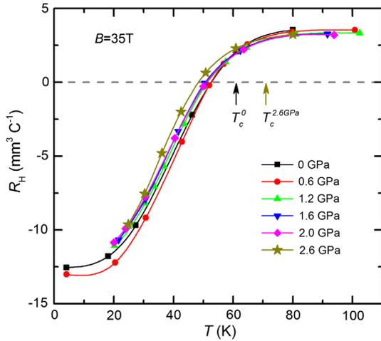
FIG. 3. Hall coefficient at  $B = 35 \text{ T}$  vs temperature for Y123 with  $n_p = 0.11$  at applied pressures of up to 2.6 GPa. The lines are guides for the eye. The two arrows mark the zero field  $T_c$  at ambient pressure and at 2.6 GPa, respectively.
