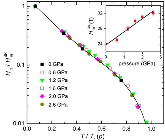
FIG. 4. Evolution of the irreversibility field  $H_{\text{irr}}$  with pressure and temperature plotted on scaled axes. The scaling field  $H_{\text{irr}}^{4\text{K}}$  was determined to best scale the data to the ambient pressure result, and its evolution with pressure is shown in the inset. The line is a guide for the eye.
