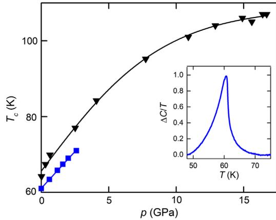
FIG. 1. Superconducting transition temperature vs pressure for the sample used in our work (the squares) compared to the behavior reported by Sadewasser *et al.* [22] (the triangles) for a similar doping. The lines are guides for the eye. (Inset) The measured heat capacity at ambient pressure of our sample close to  $T_c$  after the removal of a smooth background and scaled to unity at  $T_c$ .
