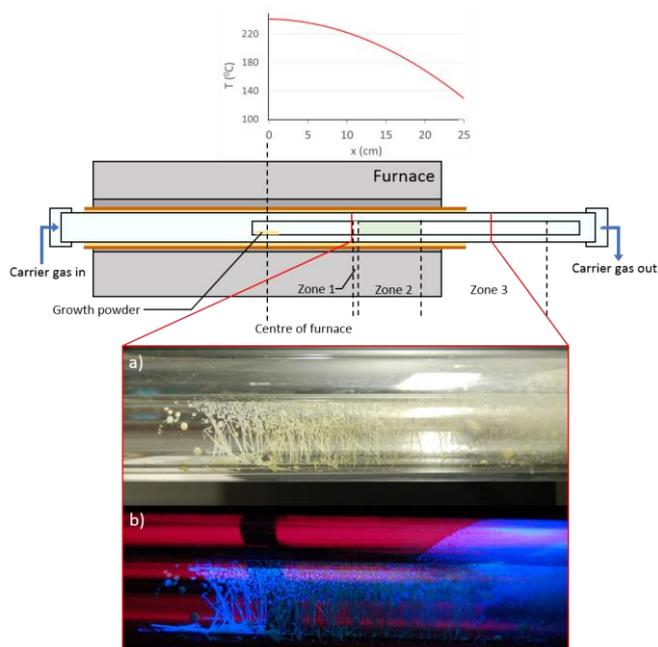
**Fig. 2** Schematic of PVT growth apparatus, including the temperature profile of the furnace. a) crystals grown in the growth tube under lab light, and b) under 365 nm UV light.
