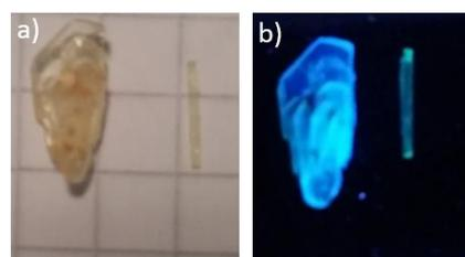
**Fig. 3** Comparison between a solution-grown crystal of form 1 (left) and a PVT-grown crystal of form 2 (right) under a) lab light, and b) 365 nm UV light. Squares are 0.5 cm<sup>2</sup>.
