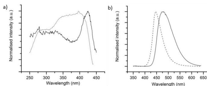
**Fig. 5** (a) Absorption and (b) emission spectra of Br-FN crystals of form 1 (dotted lines) and form 2 (solid lines).
