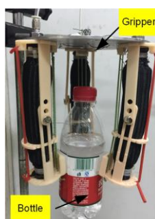
FIGURE 10. Grasping of a bottle of water using the SFLM gripper.
