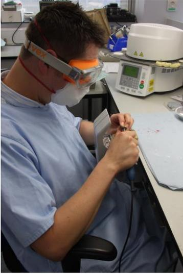
Using protective personal equipment while grinding alloys
