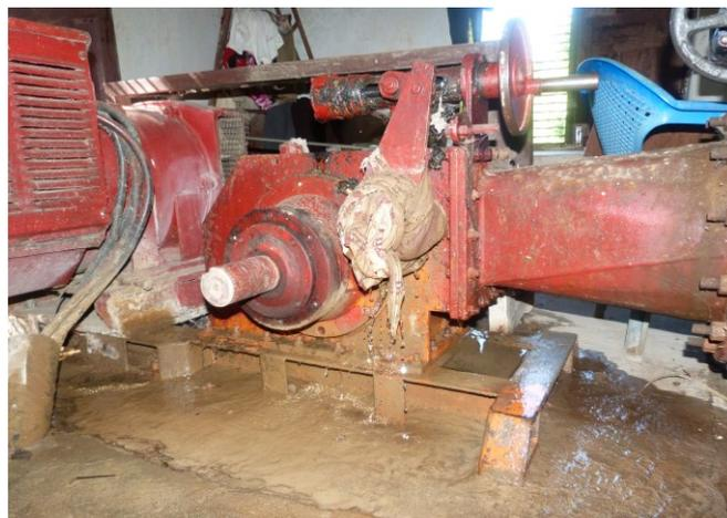
Fig. 6 Leakage from turbine casing
