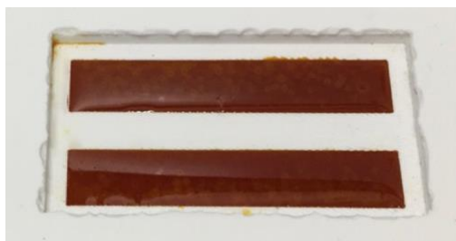
Figure S1. BMI-0 s cast in silicone moulds
