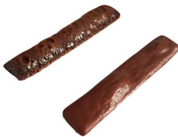
Figure S5. Porous cured BMI specimens.
