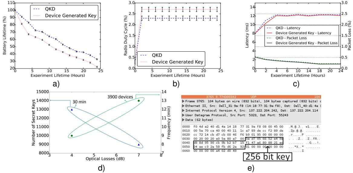
**Fig. 2:** a) RDC over 24h using the QKD key and the DKG, b) Battery Lifetime over 24h of the IoT devices using the QKD key and the DKG, c) Latency/Packet loss over 24h using the QKD key and the DKG, d) Number of keys and frequency that the devices can be served as a function of the optical losses in the two QCh cases, e) UDP response packet containing a 32byte key (Wireshark)
