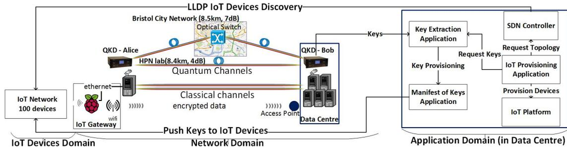
Fig. 1: Architecture of the integrated optical QKD system and IoT network
