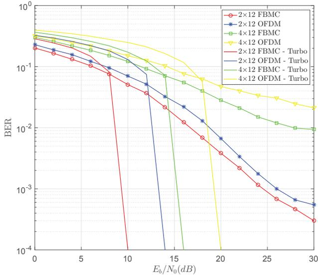
Fig. 3. BER performance of MIMO OFDM & FBMC/OQAM systems
