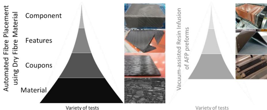
**Figure 1: Pyramid of testing approach for dry fibre AFP deposition (left) and infusion of preforms (right)**
