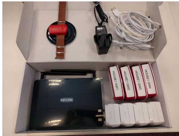
Fig. 1. The EurValve Smart Home in a Box (SHiB) kit used for the data collection.
