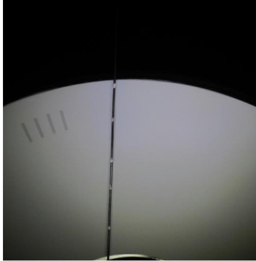
Figure 3. An example of a multiple imaging artifact, along with the vertical wire used for fixation.
