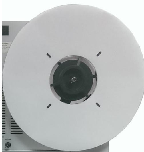
Figure 2. The white circular card attached to the tape machine, with the black lines used as the moving stimulus.
