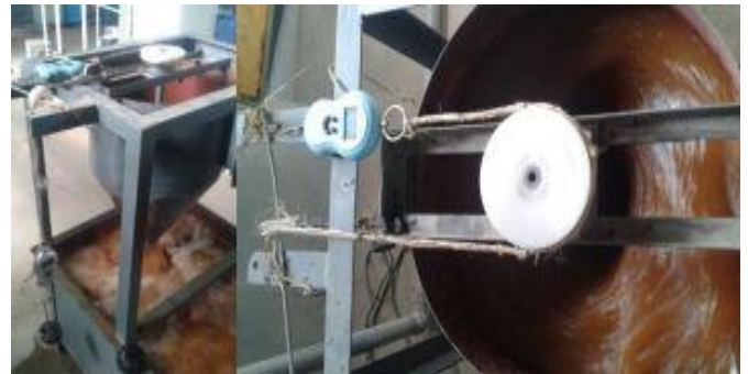
Fig.14: Prony brake dynamometer system.
