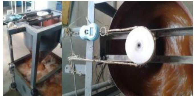
Fig.14: Prony brake dynamometer system.
