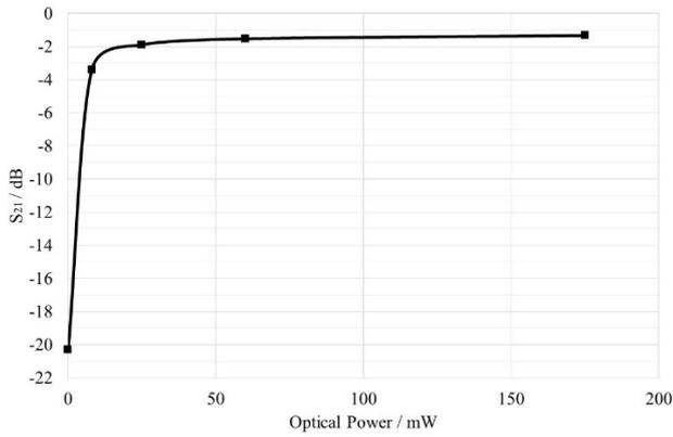
**Fig. 5.** Measured  $S_{21}$  magnitude vs. optical power for 0.4mm gap 1mm linewidth superstrate microstrip gapline at 2GHz
