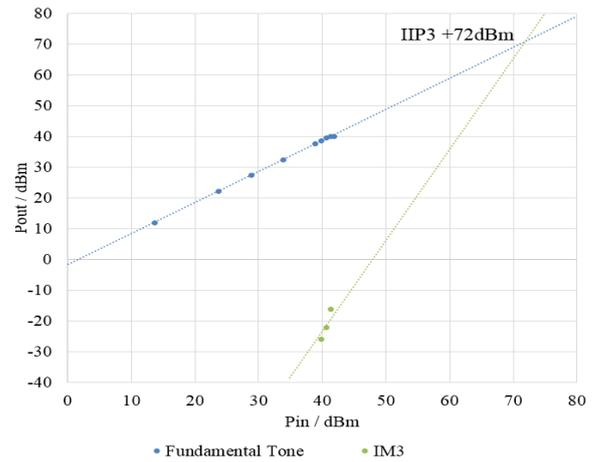
Fig. 12.  $P_{out}$  vs.  $P_{in}$  with 3<sup>rd</sup> Intercept Point at +72dBm
