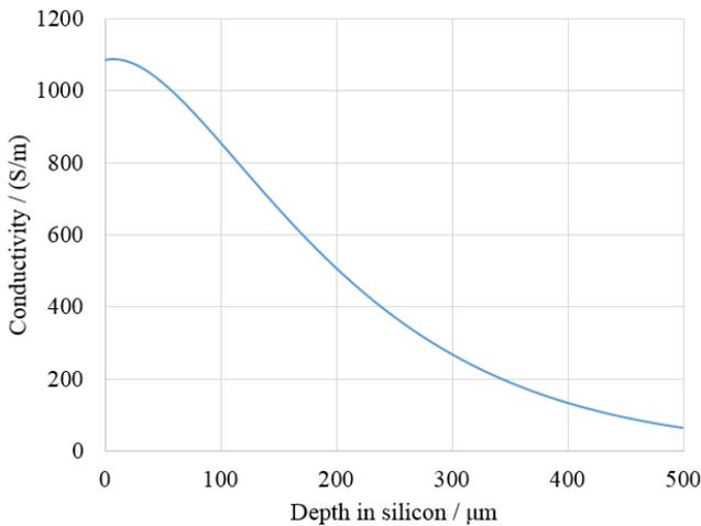
**Fig. 6.** Conductivity vs. diffusion depth in silicon superstrate
