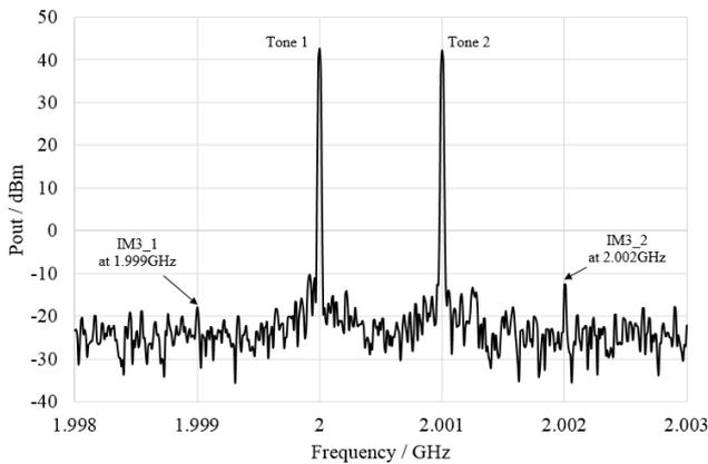
Fig. 11.  $P_{out}$  spectrum at  $P_{in}$  of +43.0dBm
