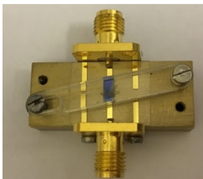
Fig. 2. Top view of superstrate microstrip gapline with bottom illumination
