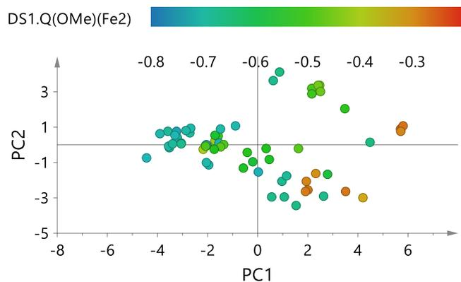
Figure 3: PC score plot (PC1 & PC2) coloured according to Q(OMe) (Fe<sub>2</sub>).
