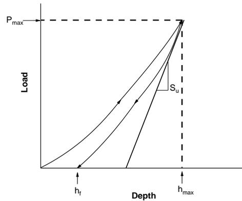
**Figure 2.** Example representation of indentation-load displacement data showing key parameters.  $P_{max}$ , peak indentation load,  $h_{max}$ , indenter displacement at peak load,  $h_f$ , final depth of the contact impression after unloading and  $S_u$ , contact stiffness of unloading curve calculated from the unloading gradient. Adapted from literature [10].
