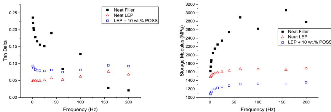
**Figure 7.** Comparison of filler, unmodified LEP and modified LEP (10 wt.% POSS) DMTA single cantilever frequency sweeps conducted under 0.1 to 200 Hz at an amplitude of 15  $\mu\text{m}$  under ambient conditions. Left:  $\tan \delta$  comparison. Right: Storage modulus comparison.
