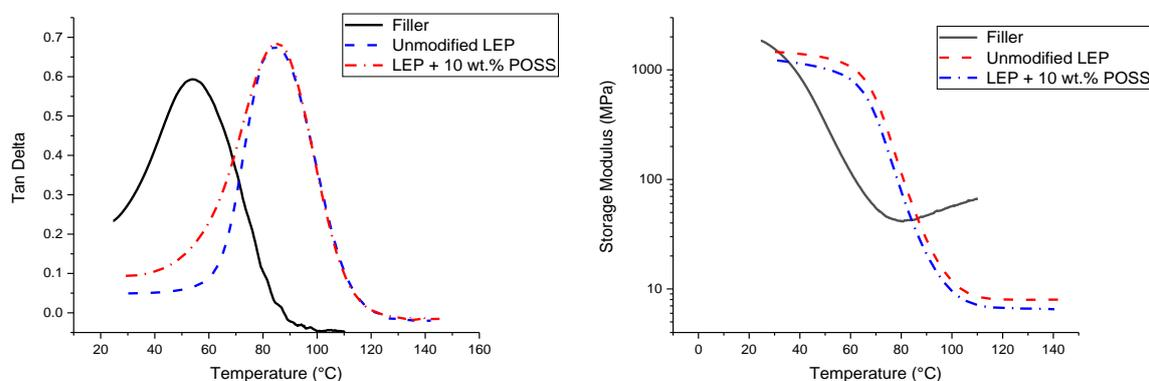
**Figure 6.** Comparison of filler, unmodified LEP and modified LEP (10 wt. % POSS) DMTA single cantilever temperature scans conducted using a 15  $\mu\text{m}$  amplitude, 1 Hz frequency and while under a dynamic scan from room temperature to 150 °C at 5 °C/min. Left:  $\tan \delta$  comparison. Right: Storage modulus comparison.
