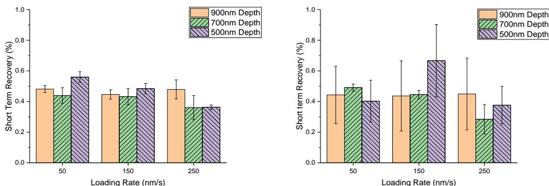
**Figure 5.** Nanoindentation of unmodified LEP and filler coated GFRP sample to investigate the effect of loading rate. Short term recovery was calculated from Oliver-Pharr analysis [19]. Left: Indentation of the LEP cross-section. Right: Indentation of Modified LEP (10 wt.% POSS) cross-section.
