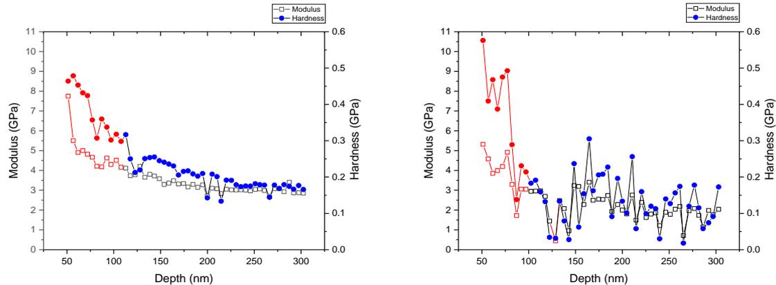
**Figure 3.** Nanoindentation of unmodified LEP and filler coated GFRP sample to investigate potential anisotropy. Modulus ( $E$ ) and hardness ( $H$ ) were determined using Oliver-Pharr analysis. Results highlighted in red are omitted from further statistical analysis. Left: Surface indentation through the LEP into the sample. Right: Indentation of cross-section of LEP film.
