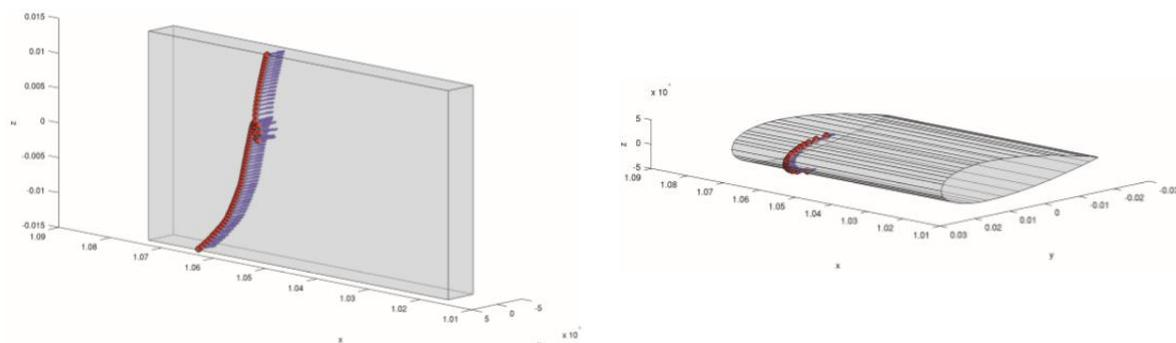
**Figure 3.** Droplet impact locations on the flat plate (left) and the aerofoil sample (right) determined computationally.
