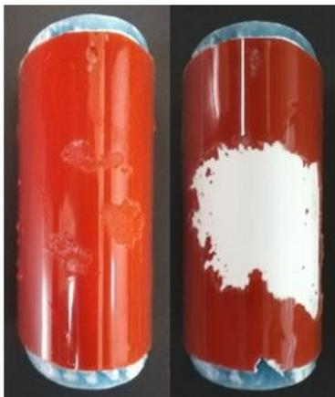
**Figure 14.** Coating samples after 20 minutes (left) and 35 minutes (right) in the ETC test rig.
