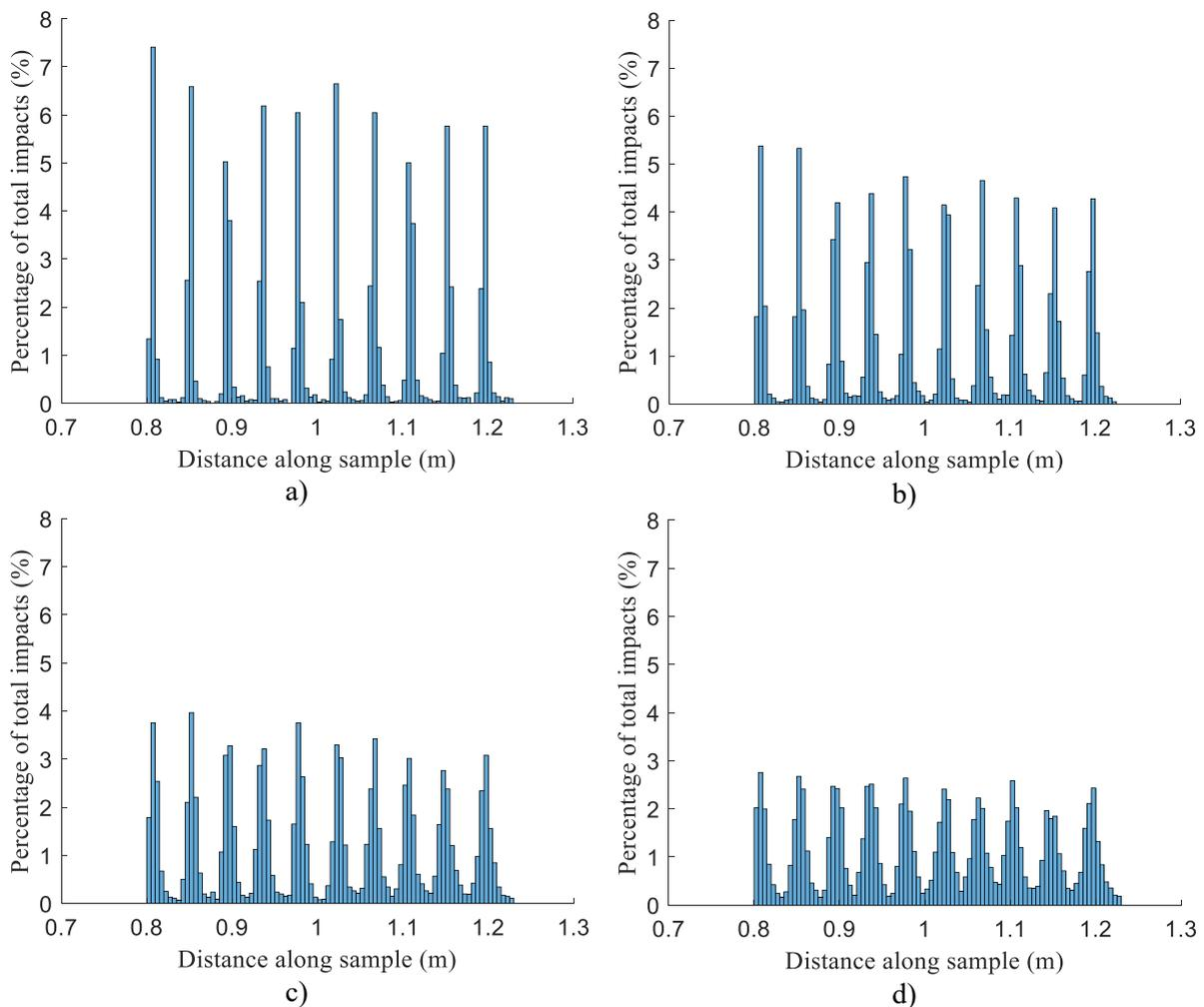
**Figure 9.** Histograms presenting the droplet impact locations determined computationally at rotational velocities of a) 800 rpm, b) 1000 rpm, c) 1200 rpm and d) 1386 rpm.
