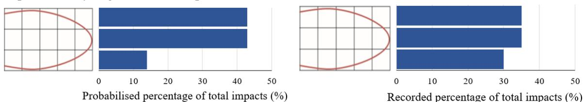
**Figure 5.** Histograms presenting the impact locations determined computationally (left) and experimentally (right) on the aerofoil sample.
