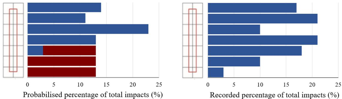
**Figure 4.** Histograms presenting the impact locations determined computationally (left) and experimentally (right) on the flat plate.
