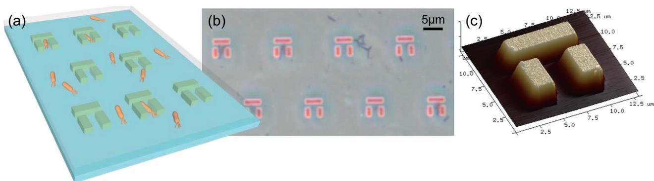
**Fig. 1** (a) Sketch of the hydrodynamic trap array. Traps (in green) are fabricated in SU8, an electron beam negative resist, on a glass slide, and are sealed with a PDMS channel to allow injection of the bacterial solution. (b) Phase contrast image of a section of a microfluidic channel and trap array, some of which are populated with bacteria. (c) Atomic force microscopy (AFM) image of a single trap on a microscope slide.
