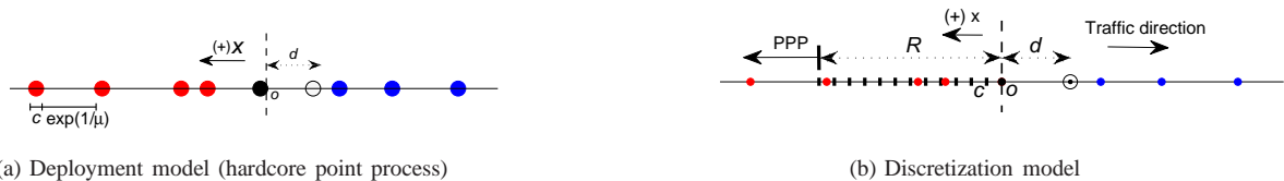
Fig. 1. (a) The vehicles are modeled as identical impenetrable disks of diameter c . Their antenna is placed at the right side of the disk. A transmitter (black disk) is conditioned at the origin and paired with the receiver (hollow disk) at x = -d . The vehicles behind the transmitter (red disks) generate interference at the receiver, while the rest (blue disks) do not. All vehicles move rightwards but the interferers are assumed in the positive half-axis to simplify the expressions. (b) The line segment c \leq x \leq R is discretized with interval equal to c . The vehicles are modeled by dimensionless points located uniformly inside the discretization intervals. For x > R the locations of vehicles are approximated by PPP.
