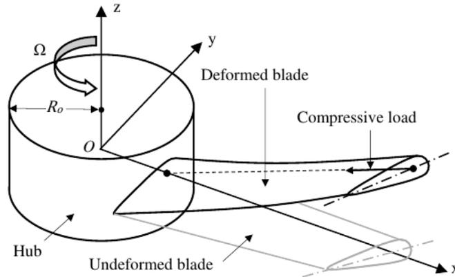
Fig. 1 Schematic of compressively loaded blade concept.
