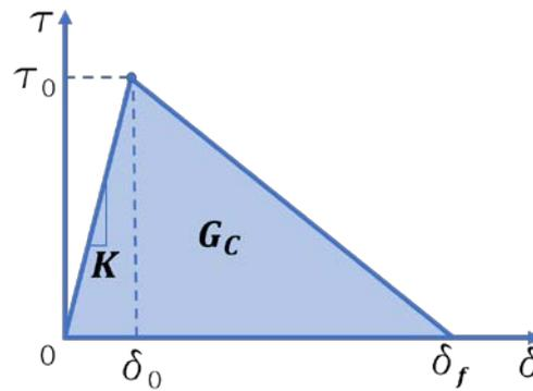
**Figure 1.** Bilinear traction separation law
