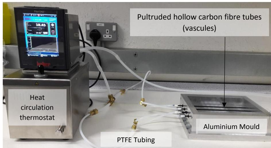
Figure 1: Lab-scale setup.
