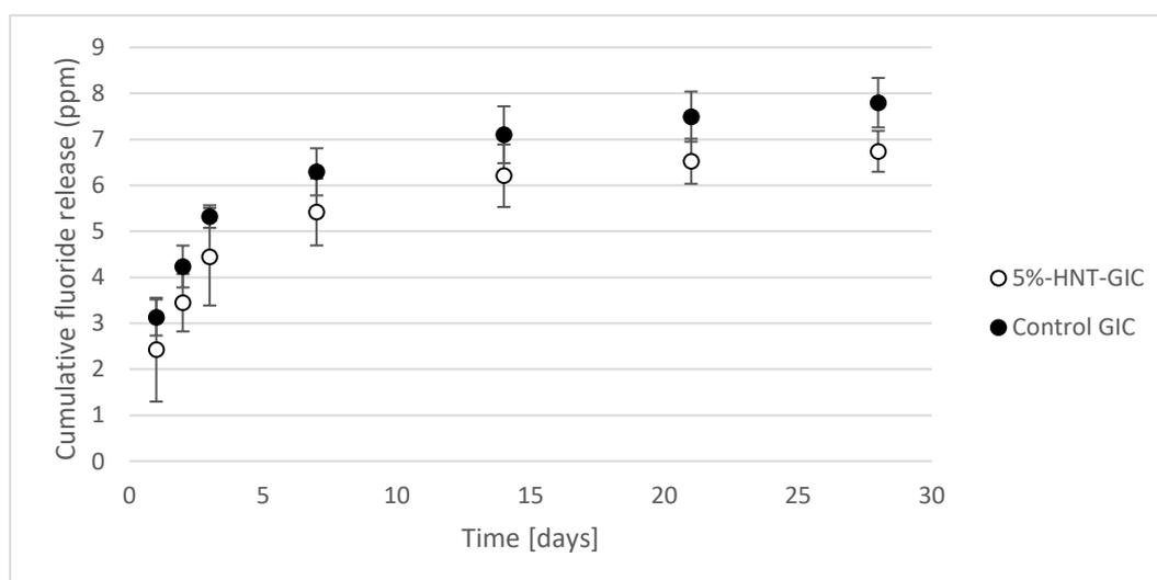
**Figure 4.** Cumulative fluoride release from control GIC (milled, no HNT, standard 4:1 powder:liquid ratio) and 5%-HNT-GIC (GIC, milled, with 5% HNT and a powder:liquid ratio of 5:1). Error bars represent standard error. Significant reductions in fluoride release were seen at days 1 ( $p = 0.0013$ ), 2 ( $p = 0.039$ ), 21 ( $p=0.0003$ ) and 28 ( $p = 2.23 \times 10^{-5}$ ).
