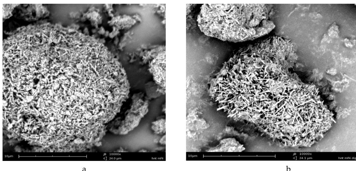
**Figure 3.** HNTs before (a) and after (b) immersion in pH 2 HCl for 15 minutes. Scale bars represent 10 μm.
