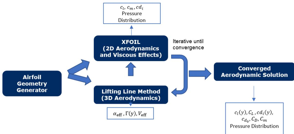
Figure 4: Aerodynamic solver algorithm
