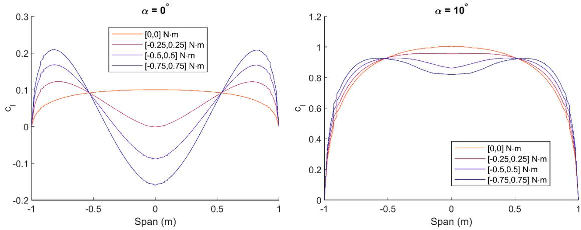
Figure 7: spanwise lift coefficient distribution for asymmetric differential actuation (i.e. equal magnitude but opposite direction) at two fixed angles of attack. The freestream flow was fixed at 30 m/s, and Reynolds number of 540000
