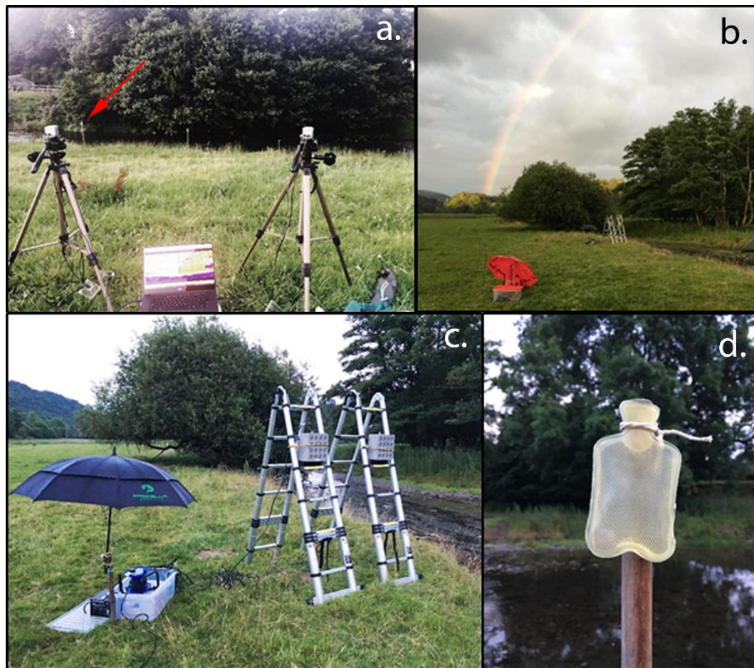
Figure 3.3 Photographs of experiment set-up at a riparian site: (a.) dual camera set-up, including red arrow indicating positioning of 15 m thermal marker at beginning of FOV and treatment area, (b.) example of speaker positioning in situ , (c) speakers positioned on ladders and (d) close-up of hand warmer used as thermal marker attached to stake on site. Photo credits L.R.V. Gilmour and S.R. Vincent.
