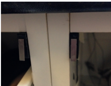
Fig. 2: Miniature snap-action switches installed in a cupboard and a drawer.
