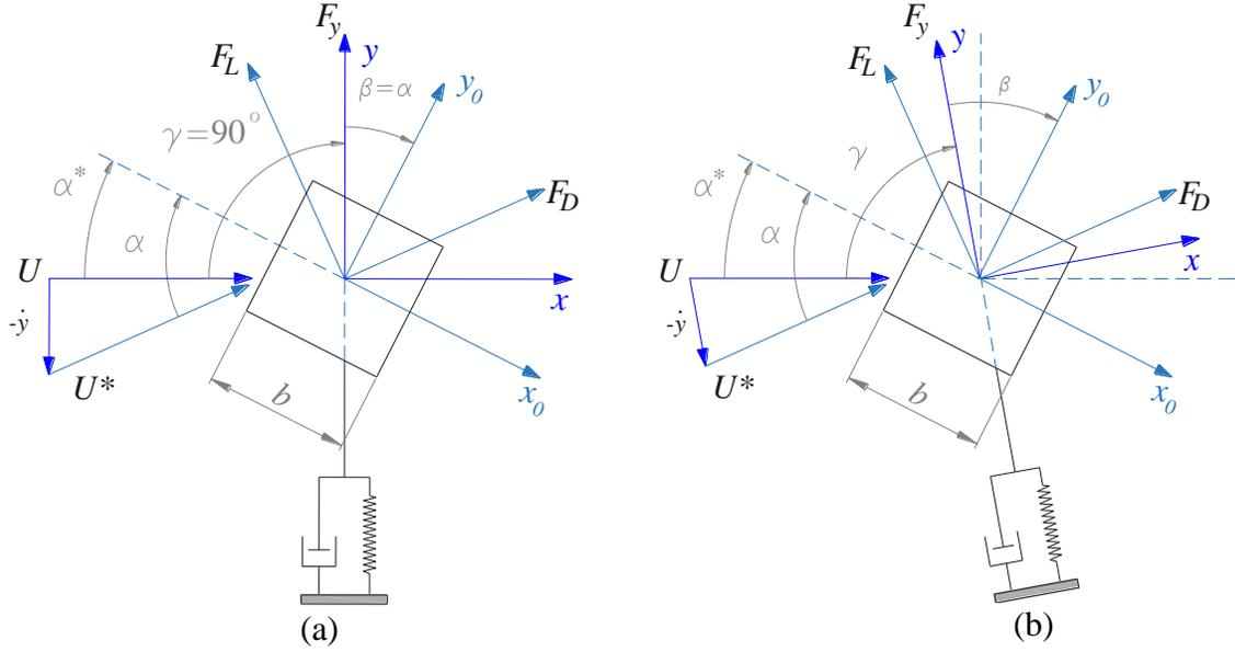
**Fig. 1** Cross-section subjected to mean wind velocity,  $U$ , indicating angles  $\gamma$  and  $\alpha$  between the wind velocity and principle axis ( $y$ ) and body reference axis ( $x_0$ ) – (a) cross-wind oscillation, i.e.  $\gamma=90$ ; (b) non-across-wind oscillation
