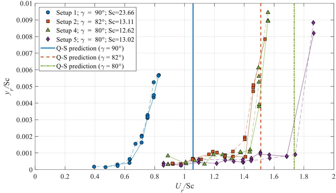
**Fig. 9** Normalized galloping amplitudes for angle of attack  $\alpha = 10^\circ$  for different orientations of the principal structural axes,  $\gamma = 80^\circ, 82^\circ$  and  $90^\circ$ ; solid lines stand for increasing wind speed, dashed lines for decreasing wind speed
