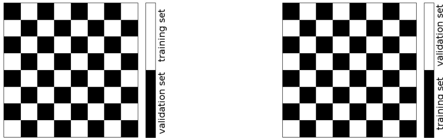
Figure 3. Training and Validation set 1 (left) and Training and Validation set 2 (right). The domain is subdivided into two subsets, according to a checkers scheme, that are used as training and validation set.
