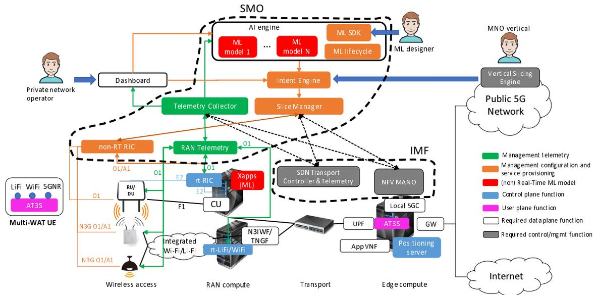
Fig. 1. 5G-CLARITY high level architecture
