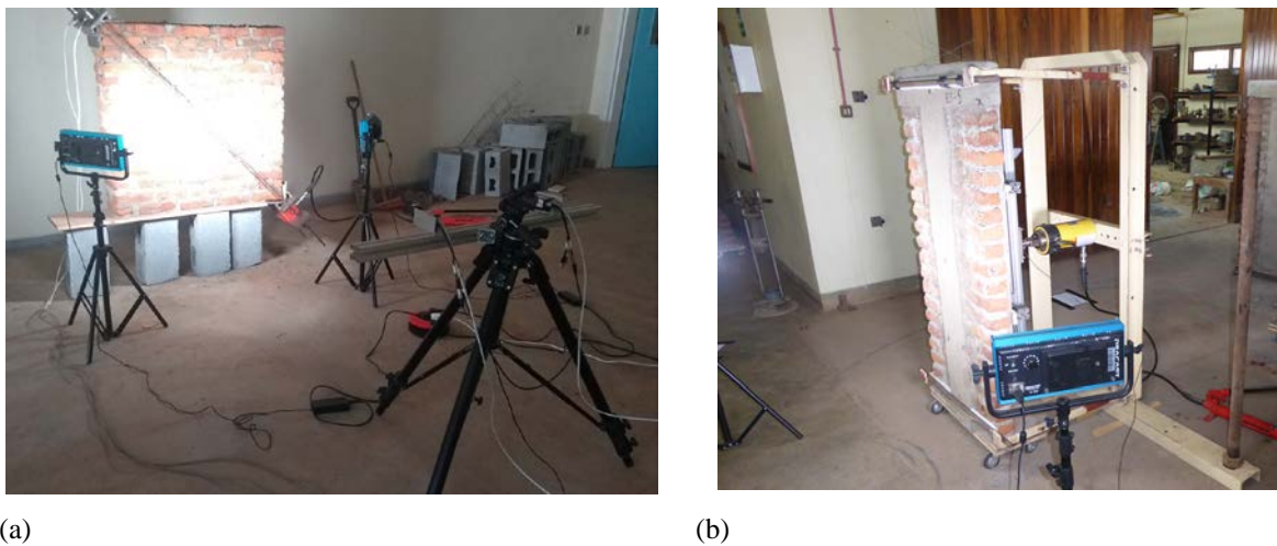
Fig. 6 – The (a) in-plane and (b) out-of-plane testing apparatus and Imetrum Vision System.
