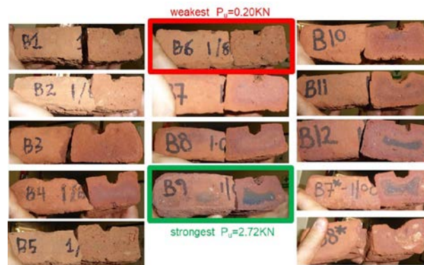
Fig. 9 – Fired clay bricks tested in flexure(/shear) (3-point bending test) from the 2019 batch.
