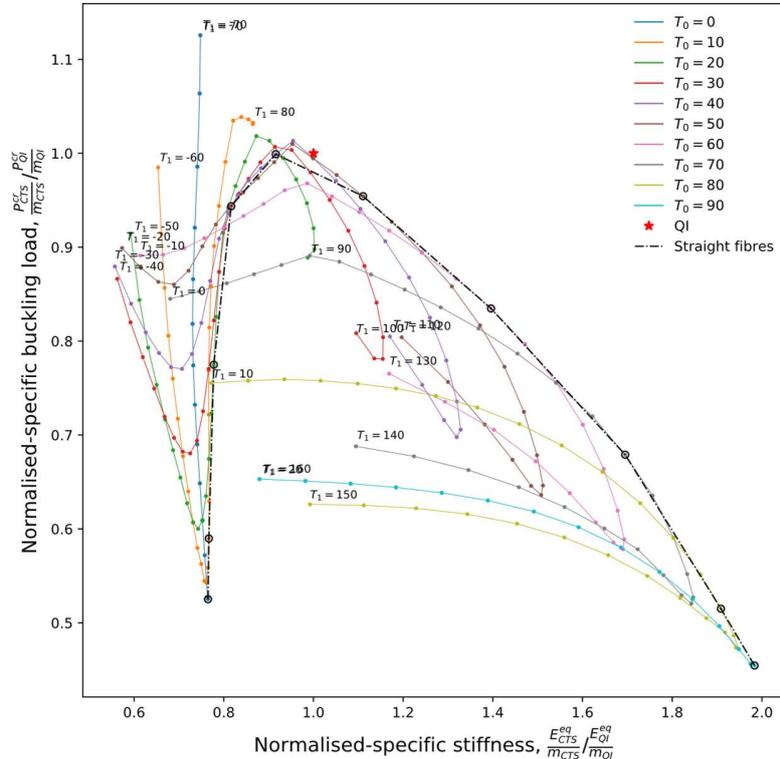
**Fig. 2 Normalised axial stiffness against critical buckling load for design 6.**
