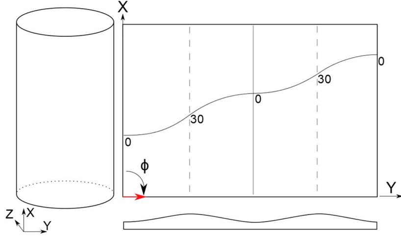
**Fig. 1 A  $90(0|30)_1^2$  lamina sheared causing two embedded-stringers to be created, shown by the cross-section.**
