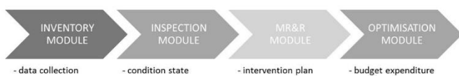
Figure 1. The modular structure of a Bridge Management System (BMS) (taken from Pregnolato 2019).
